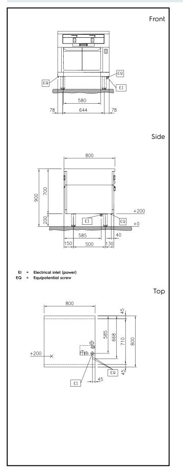
Modular Cooking Range Line thermaline 80 - 4 Zone Electric Solid Top on Warming Cabinet, 2 Sides H=700 The company reserves the right to make modifications to the products without prior notice. All information correct at time of printing.
